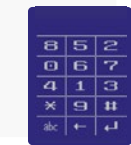
Rotating Keypad (To Prevent Surface Analysis)
